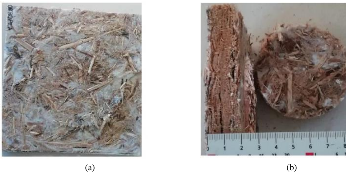
Figure 2: Final product used for the acoustic measurements: recycle of hemp (a) and corn chips (b).
